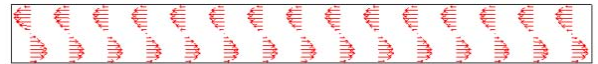
Figure 3. Velocity profile with parameters \chi_0 = 1, \tilde{\Omega} = 1, \tilde{\zeta} = \tilde{\eta} = 1, \frac{d\tilde{B}_x}{dz} = 0.00001 for non-zero spin viscosity condition ( \tilde{\eta}' = 0.01 ).
