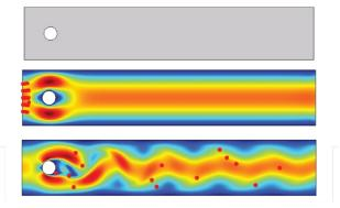
Figure 1: Fluid flow past a cylinder at different average velocities
