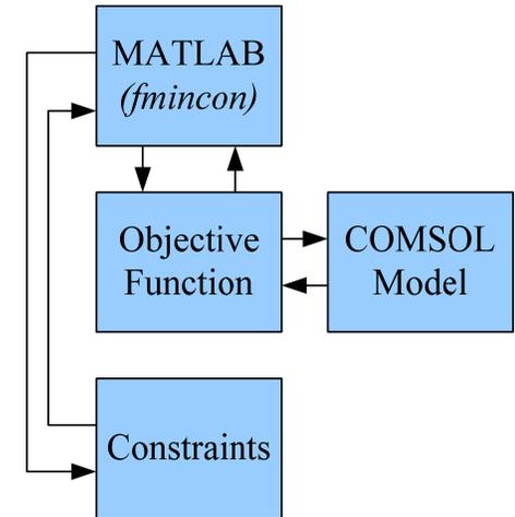
Fig. 3: Program flow of the optimization process.
