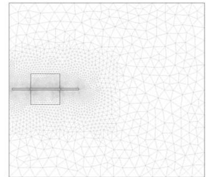
Fig. 4: Typical mesh of magnetic COMSOL model.
