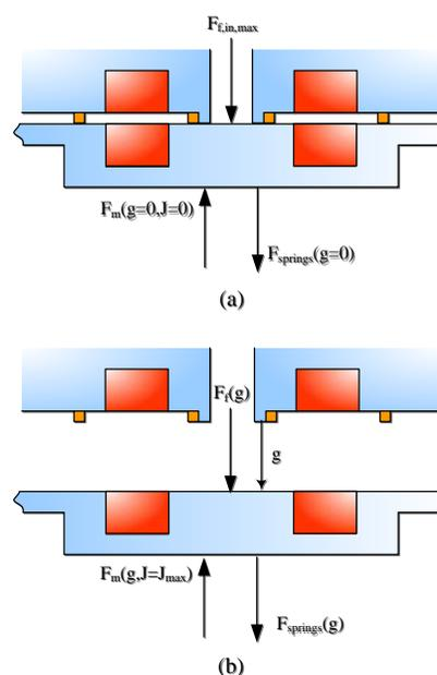
Fig. 2: Forces acting on the valve cover in the (a) closed and (b) open positions.
