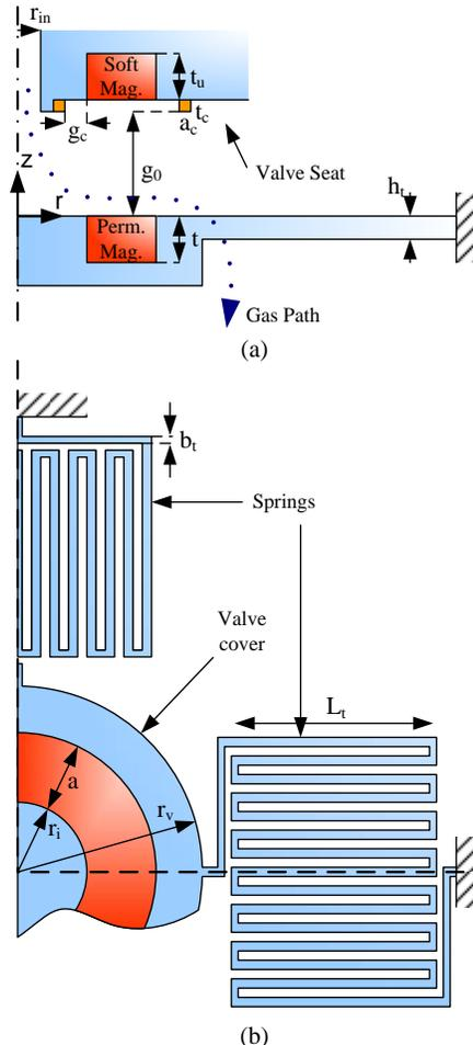
Fig. 1: Electrodynamic microvalve geometry: (a) partial cross-sectional view of mating components; (b) partial plan view of valve cover.
