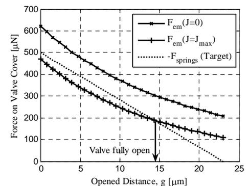
Fig. 5: Electromagnetic and spring forces acting on the valve cover.
