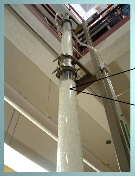
Removing CO<sub>2</sub> from air into water. Water flowing downward, gas flowing upward over packing.
