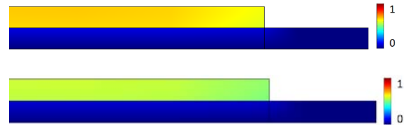
Figure 3. Normalized drug concentration after 60 hours. Top figure without enhancer, Bottom figure with enhancer. Initial enhancer concentration is 0.12 g/cm 3
