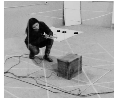
Figure 2. Sound Power Measurement Using 72 Points of Intensity Data.
