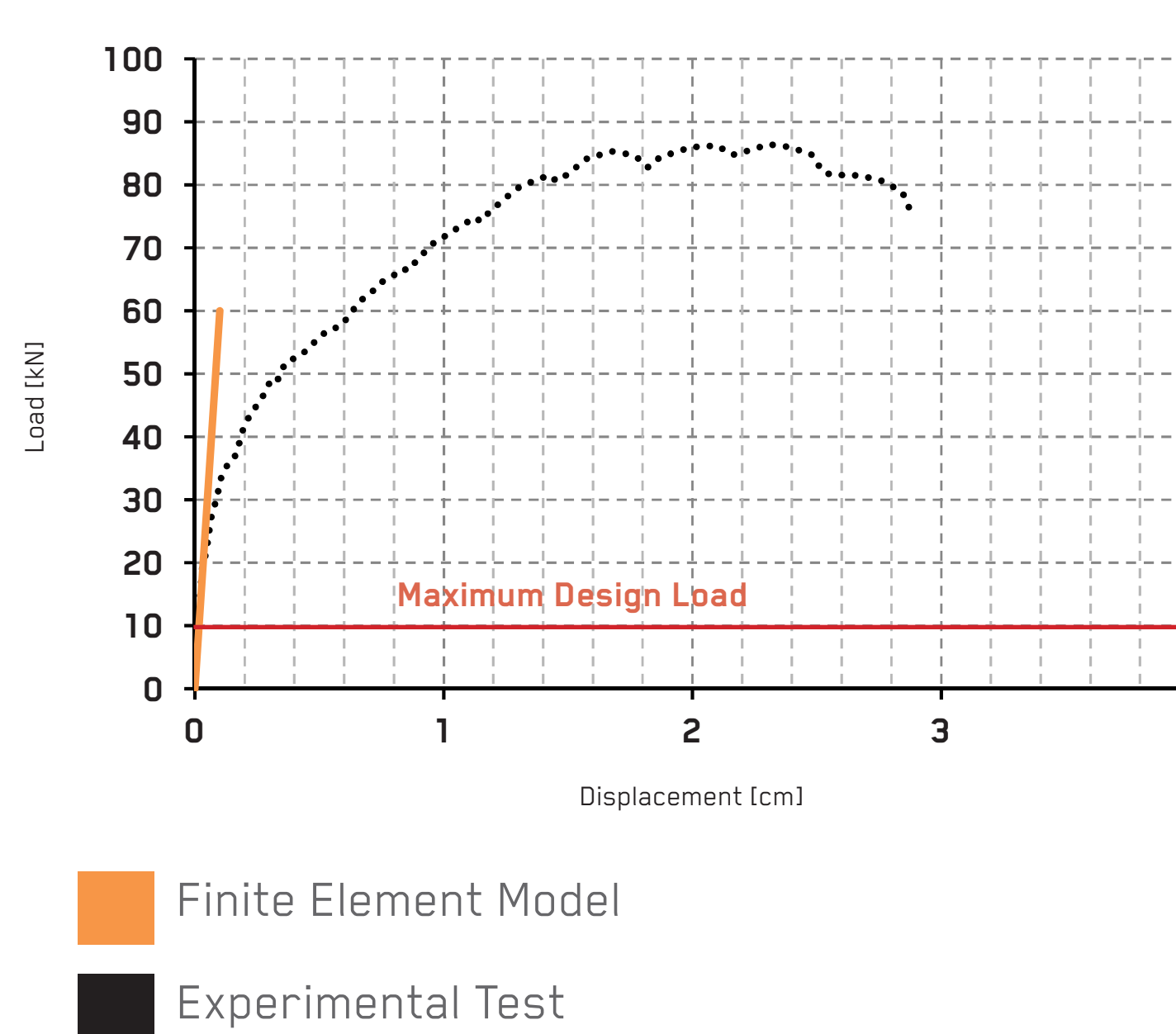
Figure 11. Comparison of Results for Pull Test (FEM and Physical Test) for GRC
