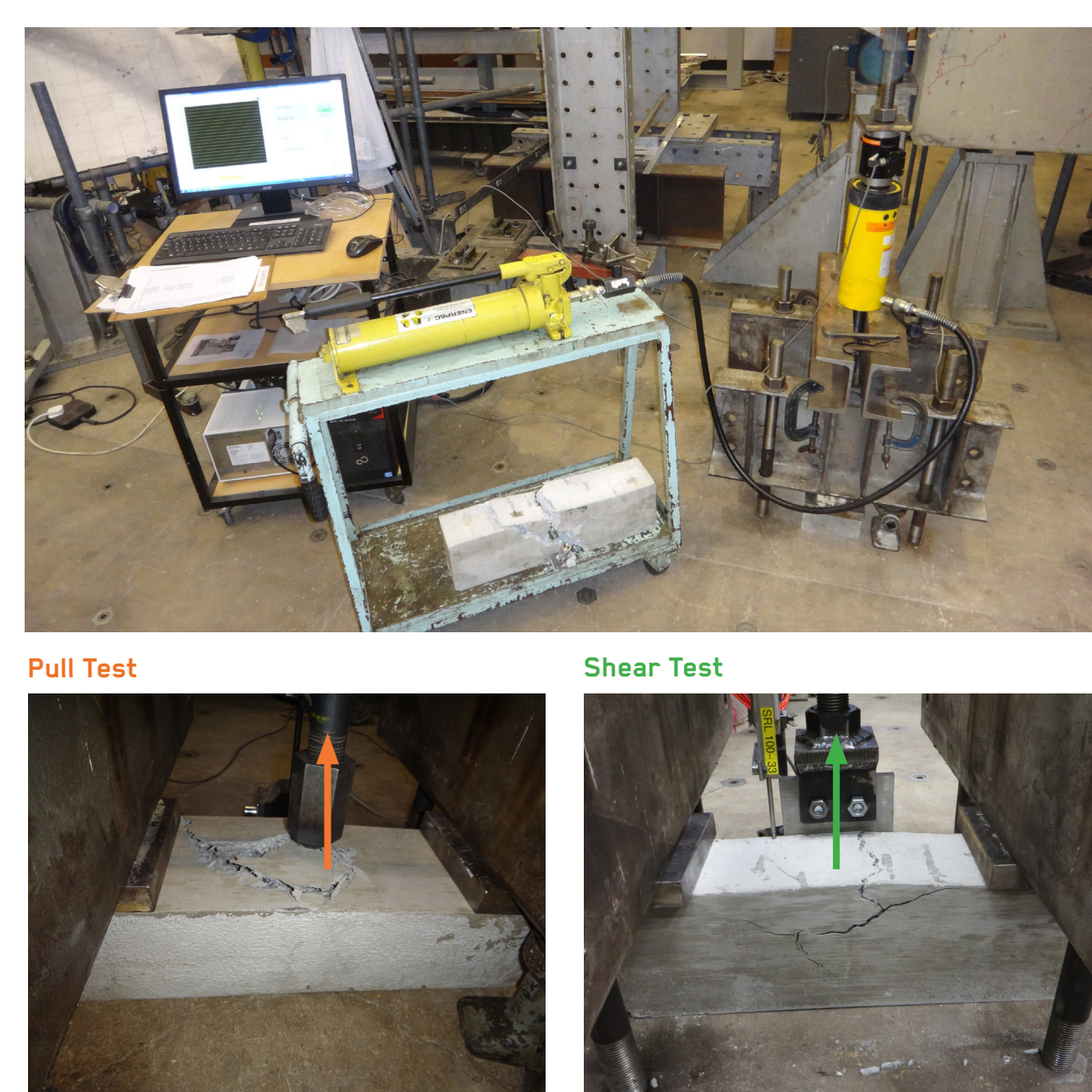
Figure 10. Testing of the Metal Connection at the University of Cambridge (UK)
