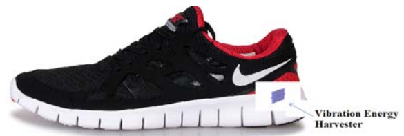
Figure 6: Shoe with vibration energy harvester inserted in its sole
