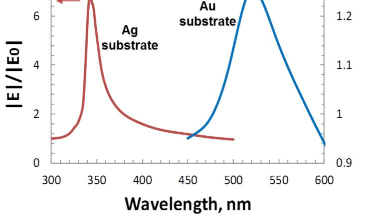
Figure 3. The maximum electric field in the gap for silver and gold substrates.
