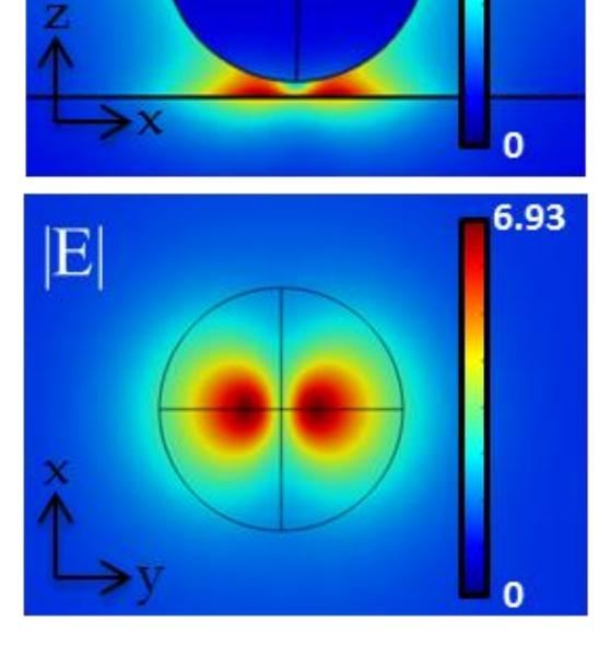
**Figure 4**. Spatial field distributions for a dielectric nanoparticle placed above a silver substrate at 343 nm.
