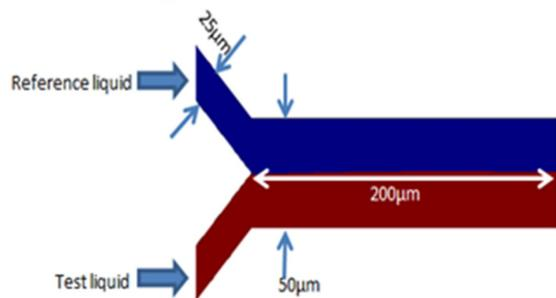
**Figure 1:** Y shaped Microfluidic Device Geometry Design
