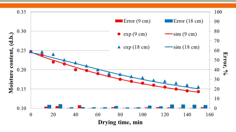
Experimental (exp) and predicted (sim) grain moisture content with drying time at different depths at  $\theta = 50$  (°C) and G = 0.22 (kg·m<sup>-2</sup>·s<sup>-1</sup>).
