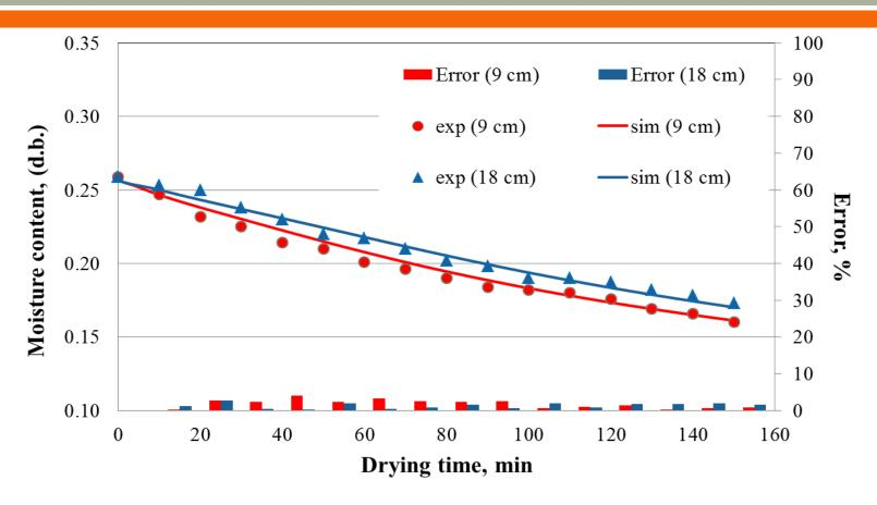
Experimental (exp) and predicted (sim) grain moisture content with drying time at different depths at  $\theta$  = 45 (°C) and G = 0.22 (kg·m<sup>-2</sup>·s<sup>-1</sup>).
