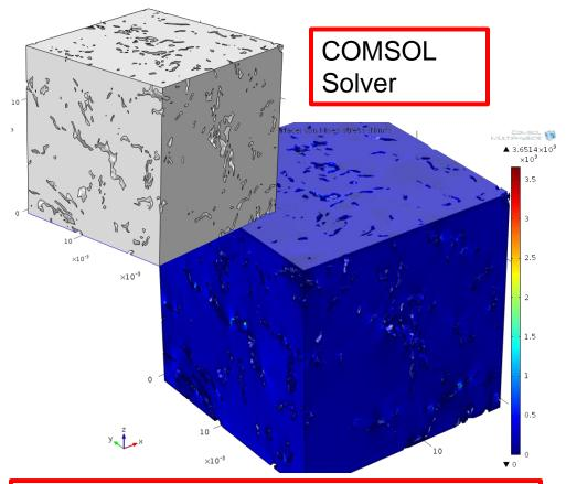
Model in COMSOL showing stress distribution. Reduction in elastic modulus and Poisson's ratio.
