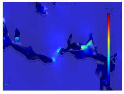
Stress concentration effect of porosity: between neighboring pores and at the edge of a single pore.
