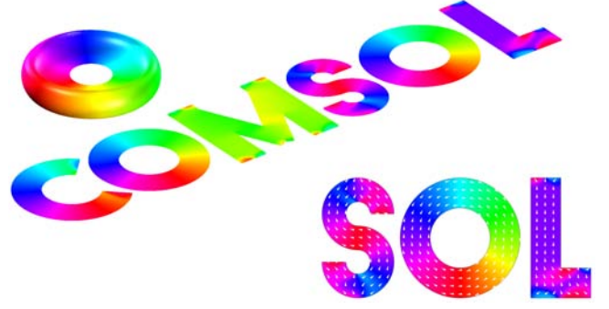
Figure 4: Two-dimensional solution of an array of thin magnetic layers. The colorcode (upper left) indicates the local direction of the magnetization distribution. On small scales, the magnetic distribution follows the shape of the geometry as shown in the inset.
