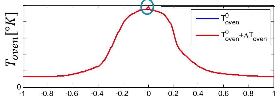
$$\Delta T_{oven}(z) = \varepsilon h(z) = \varepsilon \left( \frac{1}{\sqrt{2\pi}\sigma} \exp\left(-\frac{1}{2}\left(\frac{z-z_0}{\sigma}\right)^2\right) \right)$$
