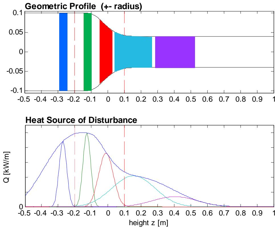
$$A\rho \left( \frac{\partial C_p(T)T}{\partial t} + w \frac{\partial C_p T}{\partial z} \right) - \frac{\partial}{\partial z} \left( Ak(T) \frac{\partial T}{\partial z} \right) = \\ 2\pi R\epsilon\sigma (T_{oven}^4(z) - T^4(z)) + Q_{dis}(z, t)$$
