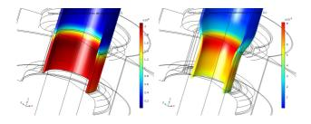
**Figure 1**: Peak compression Von Mises stress (left) and main strain (right) due to Lorentz force.
