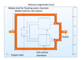
**Figure 2**: Top view of culture unit with a simulation of flushing media through the outer channels.
