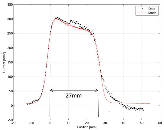
Anode current along electrode. Counterelectrode at 0.8 V. Very good agreement between experimental data and COMSOL model prediction.
