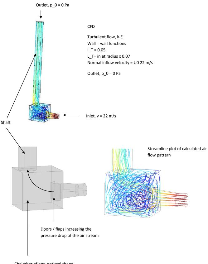
Chaimber of non-optimal shape creating turbulence and large pressure drop
